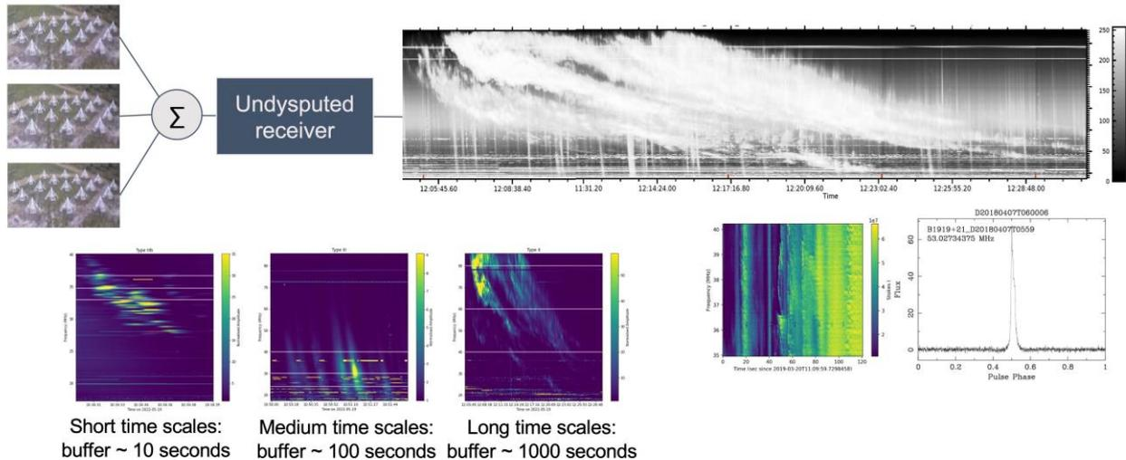
Figure A1: Schematic representing the combination of radio sensors as a sum inside Undysputed receiver which transform the raw voltage into dynamic spectra (upper right). The frequency and time resolution will restrict the access to the physical structure of the emission (here Type II & Type III bursts). A dynamic monitoring that could modify the receiver parameters can preserve the access to fine structure at small scales (bottom left).
