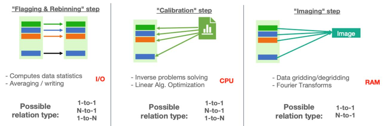
Figure C1: Description of the three main data processing steps in radio interferometry: i) cleaning the data and reducing its volume (left), ii) calibrating the data (center) and iii) imaging the whole dataset (right). One dataset (light green) contains several MS files, each one corresponding to a particular frequency.
