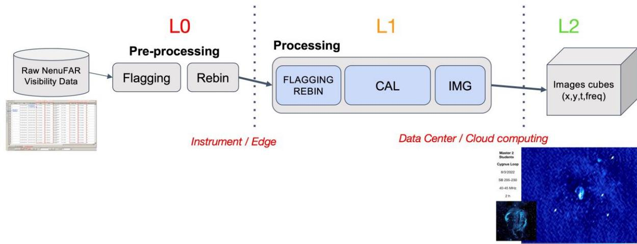
Figure C2: Generic pipeline for reducing raw interferometric data (L0, in the edge facility) to the final scientifically exploitable multi-dimensional image cubes (L2) after cleaning, compressing and calibrating the data.
