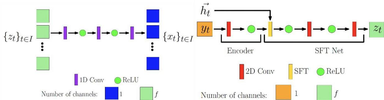
Figure D1: Proof of concept from Chiche et al. (accepted in A&A) (left) 1D net to capturing the temporal structure of the source and (right) 2D net to solve the 2D deconvolution problem.
